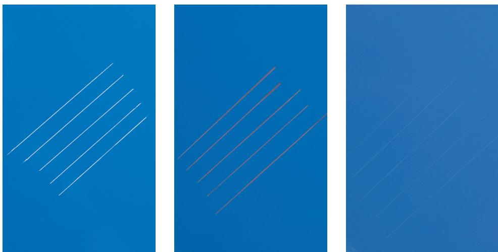
**Scratches and other** surface damage in the topcoat are not so visible if the primer shade has been selected from the same colour area as the shade of the topcoat. In the photo on the left primer shade is grey TVT 4004, in the middle red TVT 4000 and on the right blue TVT 4011. The shade of the topcoat is blue RAL 5015 for all of the panels.
