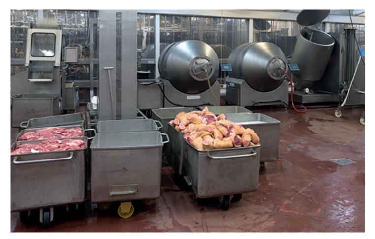
Fontefloor PU Cem is a multi-component, polyurethane concrete floor coating system. Coated surfaces are non-slip under wet or dry conditions. The system dries to a matt finish, and is available in five colors to create a clean, professional look.
